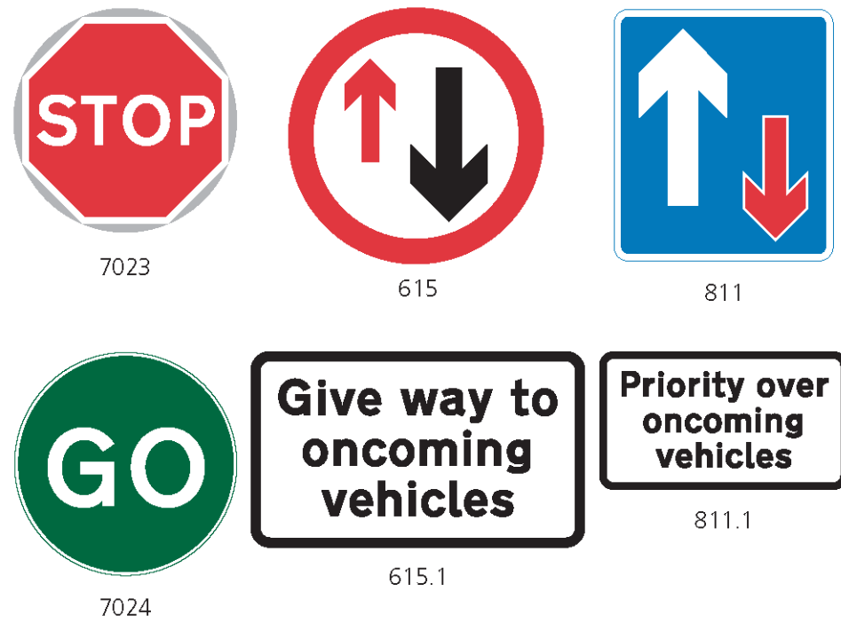
Figure 3.5: Manually Operated Stop/Go Signs and Priority Signs.
